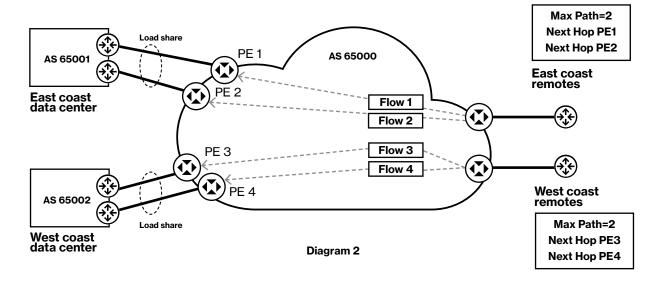
Unique BGP routes based upon originating AS number. Backbone IGP determines which data center for load-share.
